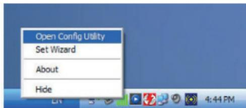
2. The configuration utility will scan for wireless networks within range. Click "**Refresh**" to refresh the list of available wireless networks. To join a particular network that displays, select it and click "**Add to Profile**".
