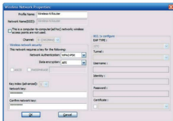
**NOTE:** For WPA/WPA2 networks, you need to select the correct encryption type, as well as (AES or TKIP). These settings depend on how the wireless network is set up. Only the owner of the wireless network can provide the required information.
