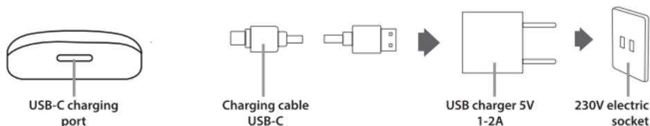
The device should be charged for about 2 hours. The LED screen will show the charge level until the letter F is displayed, which indicates that charging is complete.
